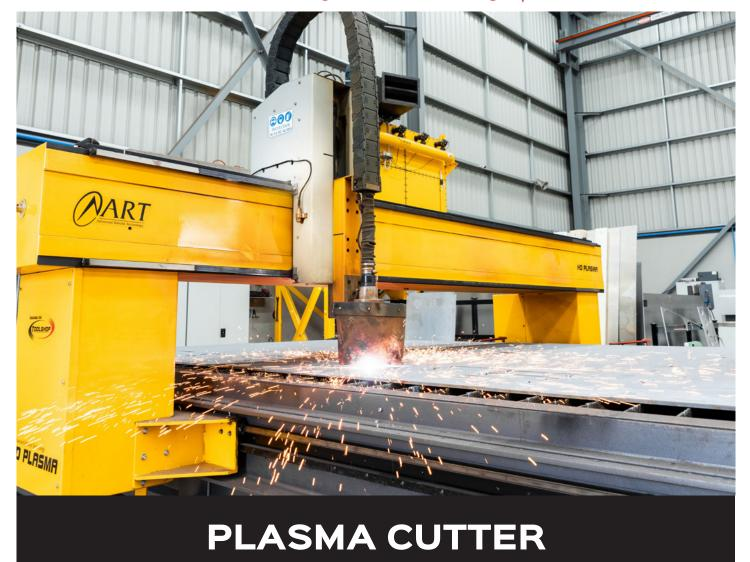
Sloanebuilt customers benefit with our new plasma cutter with quicker build times and lower costs thanks to the quicker cut times, more precise workmanship, and near-perfect micro-burr free cutting results. Our Plasma cutter helps our customer get their products at a quicker rate, for a lower cost and a more refined finish to outlast competitors.
